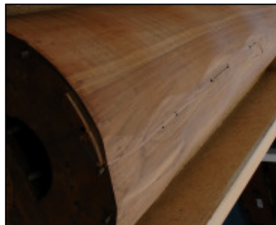
Gaps in body shell: reinforced ribs (> equipment !); fillings; planed centre part; doubled and shaped.
