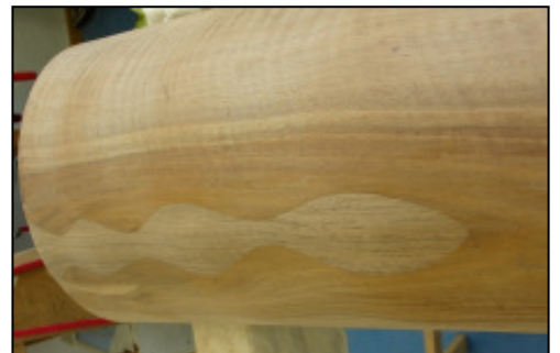
Gaps in body shell: reinforced ribs (> equipment !); fillings; planed centre part; doubled and shaped.
