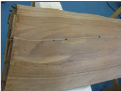
Gaps in body shell: reinforced ribs (> equipment !); fillings; planed centre part; doubled and shaped.
